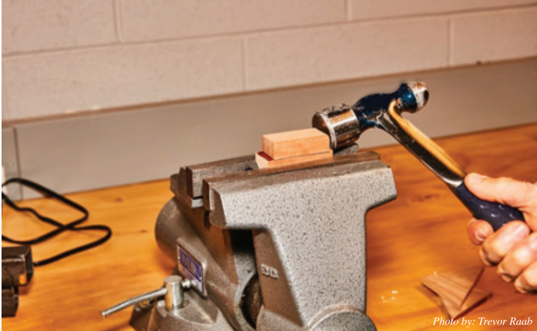
We glued together two pieces of cherry with super glue and after letting the sample cure for two hours, clamped it in a vise and hit it with a hammer. The wood failed, but the super glue did not. BSI Insta-Cure
